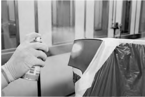
The UV-cured primer is sprayed to cover the damaged area.
