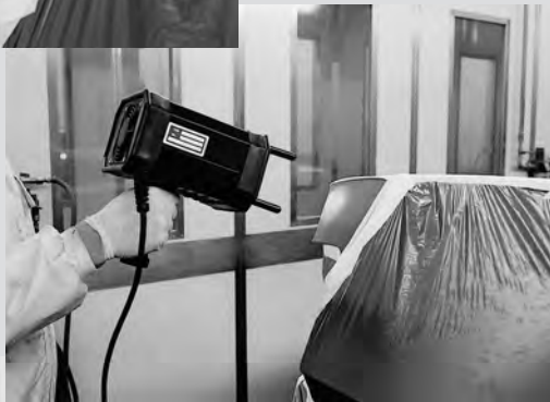
A low-energy UV lamp is used to cure the primer.
