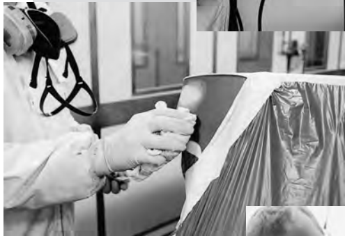
A low-energy UV lamp is used to cure the primer.
